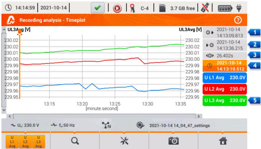
Fig. 25. Recording analysis - timeplot.
