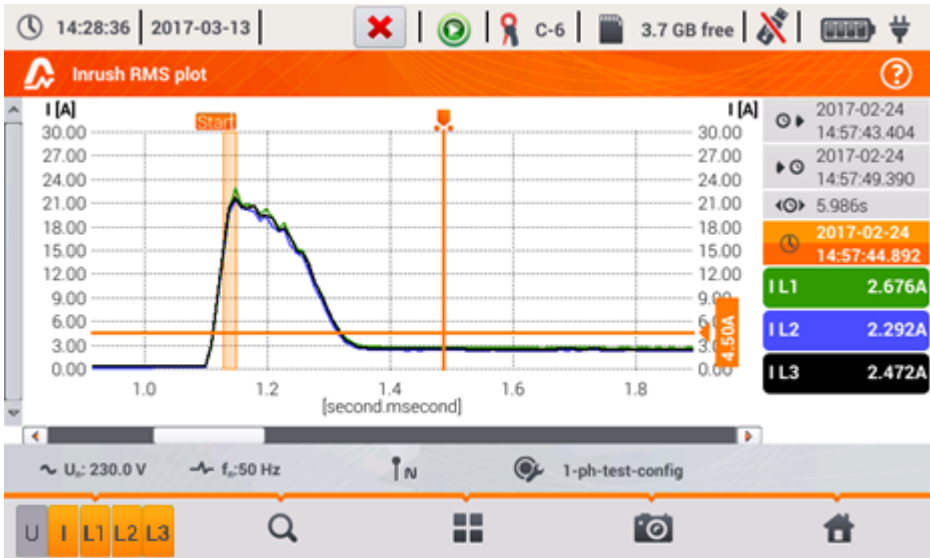
Fig. 43. Inrush current analysis – Inrush RMS plot.
