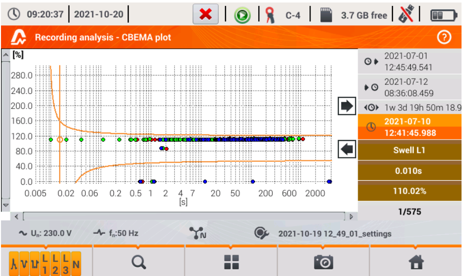
Fig. 32. Recording analysis - CBEMA graph.
