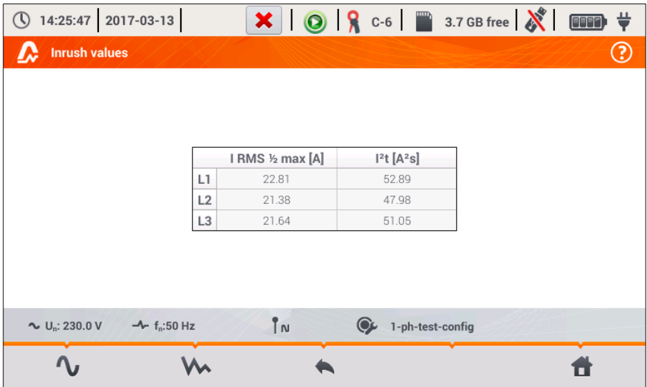
Fig. 44. Inrush current - characteristic parameters.
