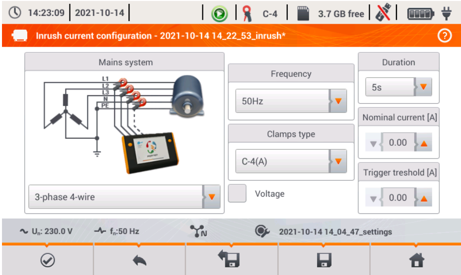
Fig. 39. Inrush current configuration screen.
