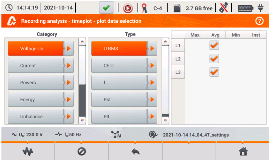
Fig. 24. Recording analysis - selecting parameters for the timeplot.
